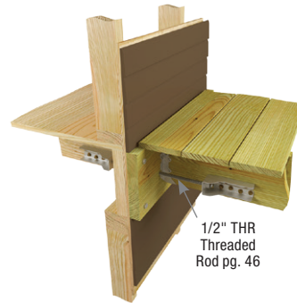
Typical DTB-TZ deck to ledger installation
