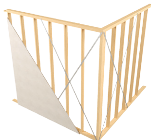
Typical RWB/WB installation
