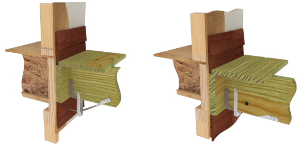
Typical ADTT-TZ full extension installation Extended Installation
