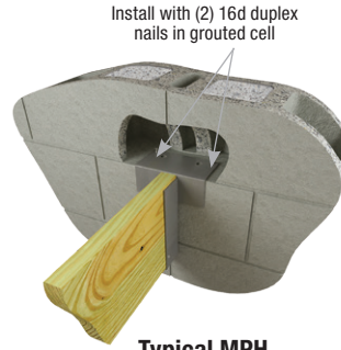
Typical MPH single-ply installation
